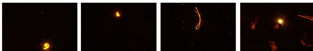
Figure 4: Documentation and staining of filters, polymer identification via fluorescence microscopy
